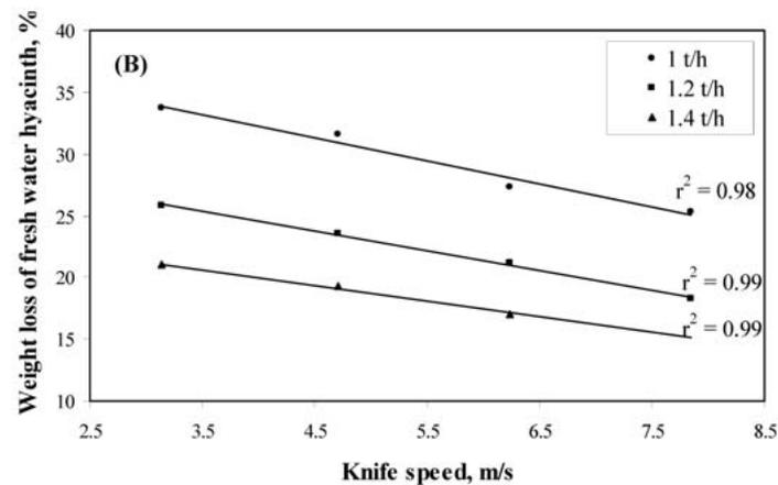
Figure 3. Effect of knife speed on chopping of water hyacinth at different feed rates (A) reduction in specific volume, %; (B) weight loss of fresh water hyacinth, % initial specific volume of freshwater hyacinth, 8.25 m<sup>3</sup>/t; initial weight of fresh water hyacinth sample, 15 kg.
