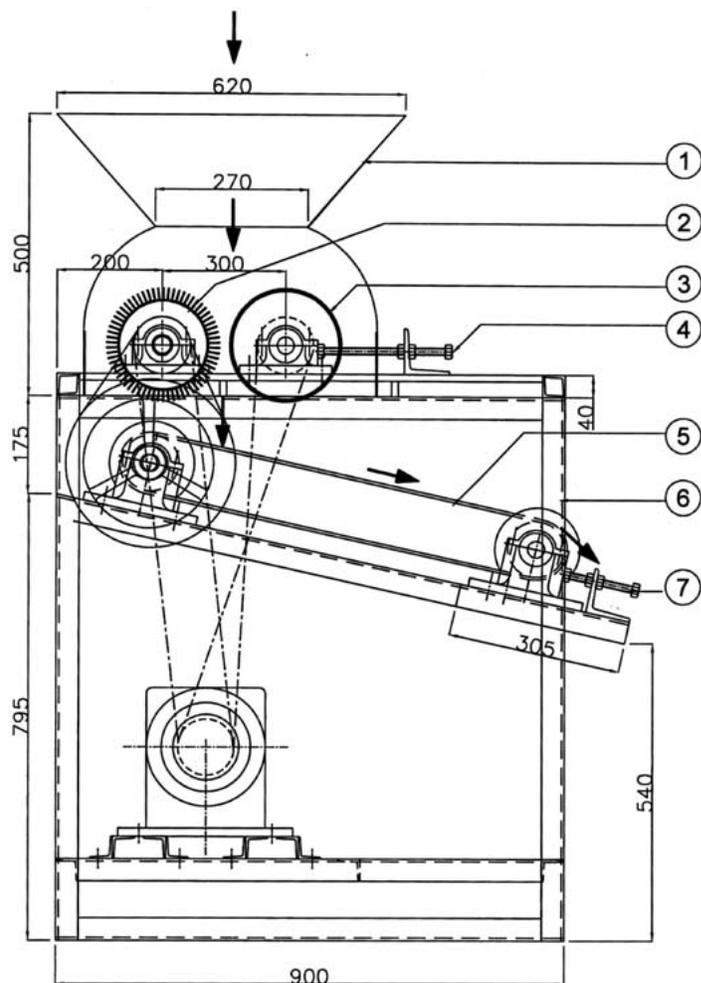
Figure 1. Water hyacinth chopper cum crusher: (1) hopper; (2) cutting roller blades; (3) pressing roller; (4) roller gap adjustment screw; (5) conveyor belt; (6) frame; (7) conveyor belt tension screw; all dimensions in mm.
