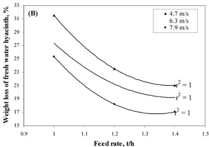
Figure 2. Effect of feed rate on chopping of water hyacinth at different knife speeds (A) reduction in specific volume, %; (B) weight loss of fresh water hyacinth, % initial specific volume of fresh water hyacinth, 8.25 m<sup>3</sup>/t; initial weight of fresh water hyacinth sample, 15 kg.
